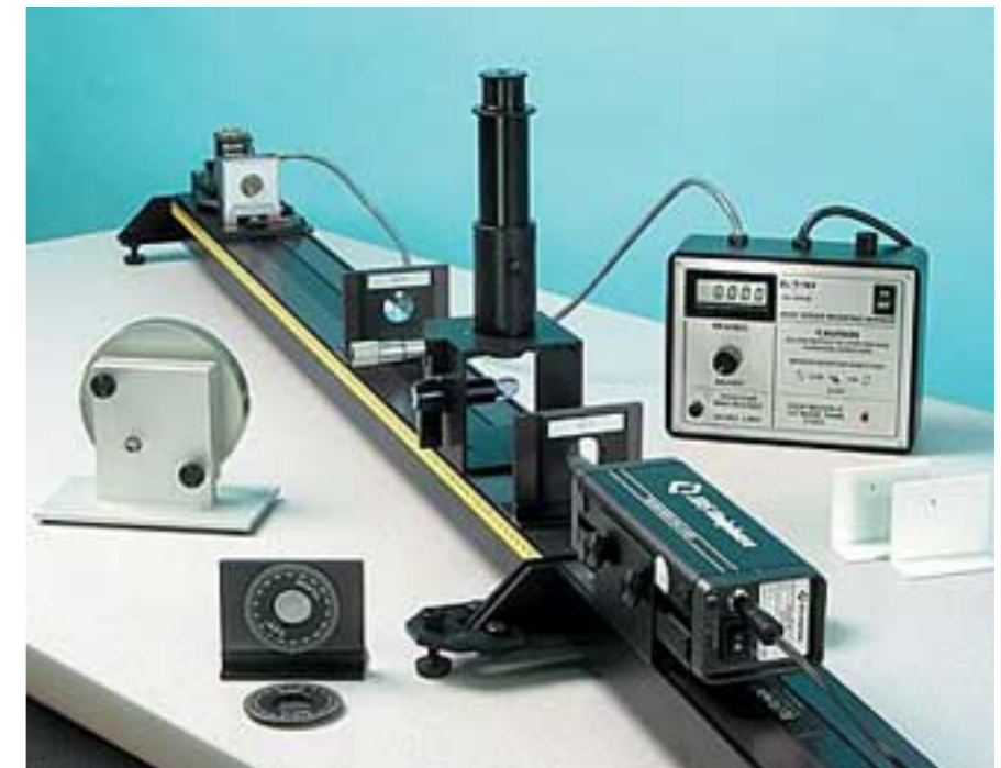
PASCO Speed of Light Apparatus
